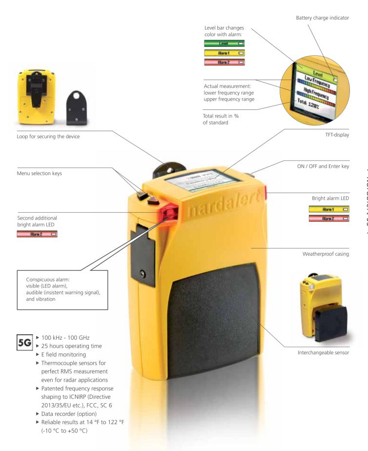
Nardalert S3 is a handy warning device that is ideal for wearing on your belt or clipped to a harness. Two different types of clip allow it to be attached to textiles or belts with equal ease. The warning lights and the display are on the top of the device so that they can be seen at a glance.
